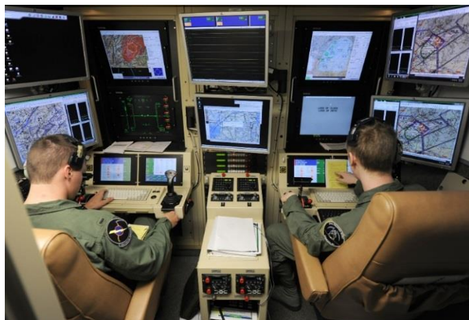
Unmanned aerial vehicle ground control station color displays. Source: DIMOC.
