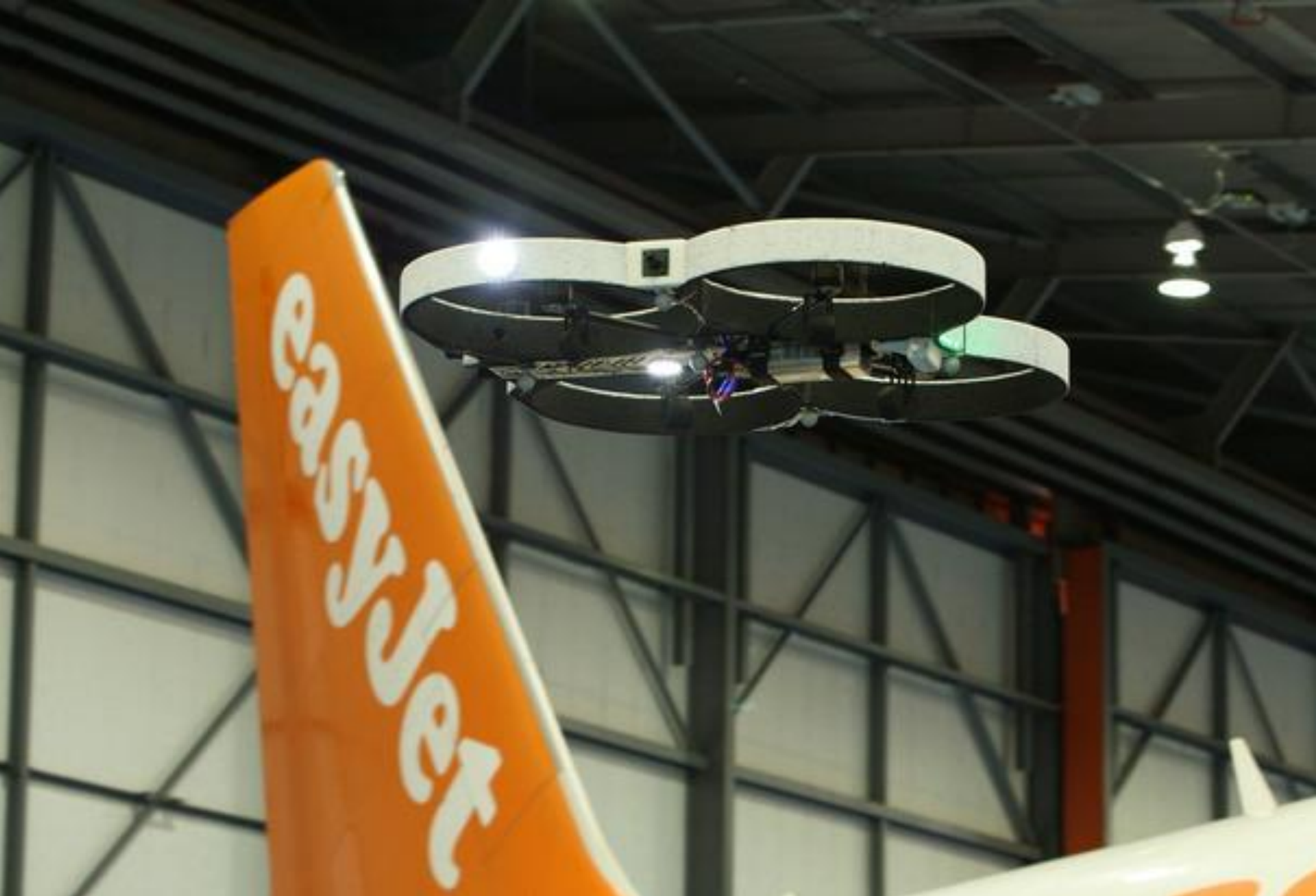
UAV used by EasyJet for fuselage inspections
