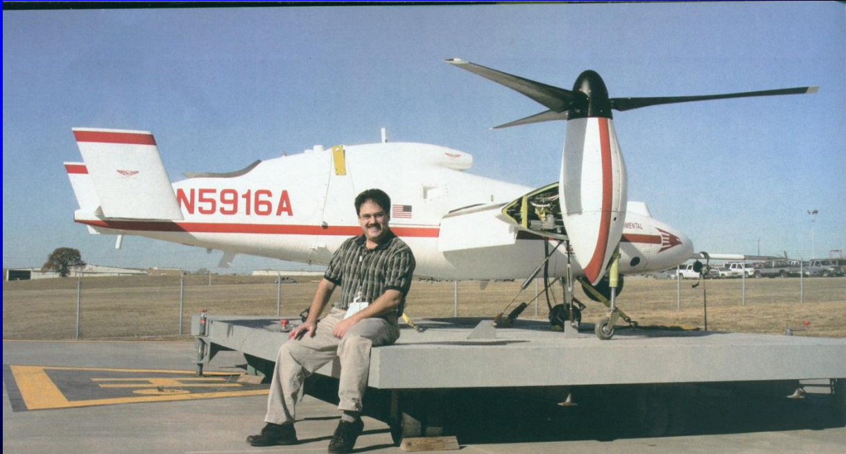
FAA Aviation Safety Inspector Marcello Mirabelli with the Bell TR918. Vehicles like this are now called unmanned aircraft systems (UASs). The Bell TR918 was developed for commercial use and certified by FAA.
